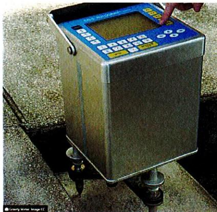
Figure 1: Gravity Survey
